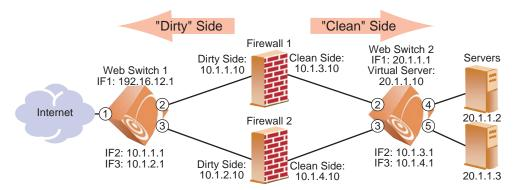
Figure 13-4 Basic FWLB Example Network
